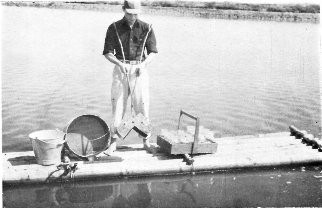
Fig. 1. A modified Ekman dredge for the quantitative study of bottom organisms in milkfish ponds has been designed and was used in the past four years. This apparatus is very efficient and convenient for use in shallow waters with hard bottom mud.
