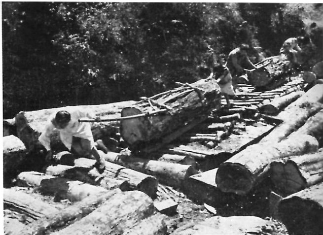
Logs are cut short (usually 2 meters) and transported on wood sled pulled by man power.
