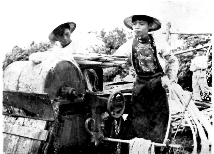
Decortication of sisal leaves with an Ikeda type decorticator.
