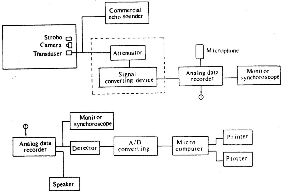
Fig. 2. Arrangement and block diagram of the acoustic system.
