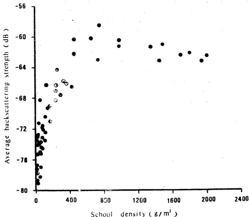
Fig. 6. Relationship between average backscattering strength and average density of simulated school.
