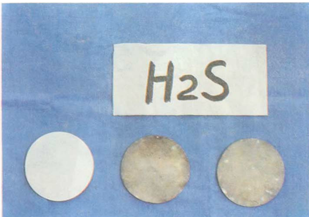
Fig 4: Detection of hydrogen sulfide in a poorly drained paddy field of an acid sulfate soil by lead acetate-treated filter paper.
