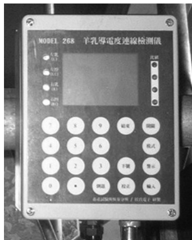
Fig. 2. The electrical conductivity meter for goat's milking machine.
