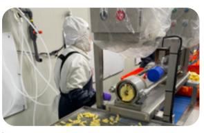
Pineapple processing: Through automated cutting of pineapples into cubes, this processing plant can size the finished products to meet the specific needs of clients.
