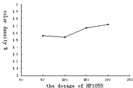
Fig.4 The effect of different HP1055 dosage on color density
