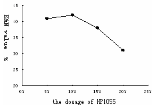
Fig.2 The effect of different HP1055 dosage on K&N value
