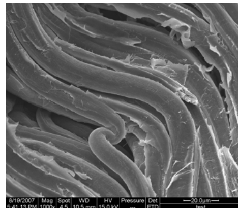
Fig. 6 The wood fiber of compressed wood on the drive section.
