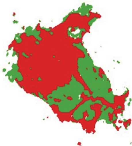
圖 13 九份二山崩塌地滑落及堆積區劃分 Fig.13 Delineation of collapse and deposition sites at Chiufengershan landslide
