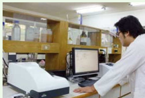
奈米微晶-粒徑分析儀 Analysis of nanoscale crystallites using a laser particle size.
