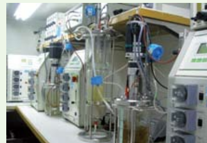
利用生物反應器生產二次代謝物 Valuable secondary metabolites are produced in a bioreactor.
