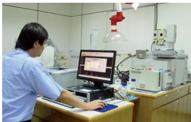
氣相層析-質譜儀分析 GC-MS analysis of the extractive components.
