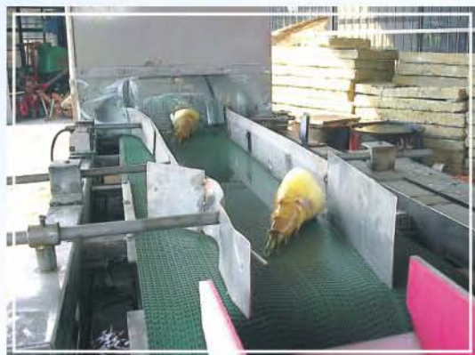
●綠竹筍清洗分級機清洗情形
