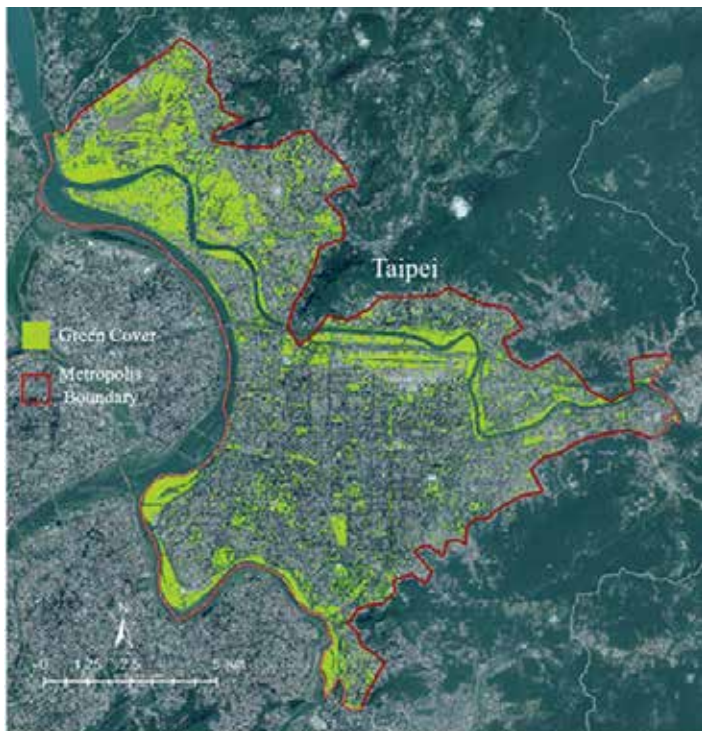
台北市都會區綠地覆蓋分布圖，底圖為2019年福衛五號正射影像鑲嵌圖。 The green cover map of the metropolis of Taipei City, the base image was a mosaic of Formosat-5 imagery collected in 2019.
