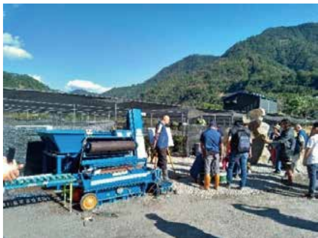
南投特作18班紙筒自動填土實機示範。 Demonstration of the automatic earth filling machine for the Paperpot at 18th forest compartment for special crops in Nantou County.
