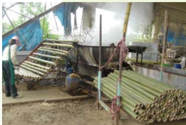
桂竹圓竹表面除污及除油處理。 Surface cleaning of Makino bamboo culms.
