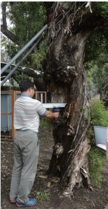
ArborSonic 3D及RESI F500-SX對於木材材質皆具備良好檢測能力。 ArborSonic 3D and RESI F500-SX are well tested for wood.
