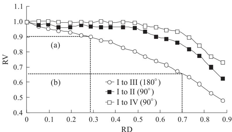
Fig. 4. Relationship of the relative velocity (RV) and the relative hole diameter (RD) for a disk with a central hole.
