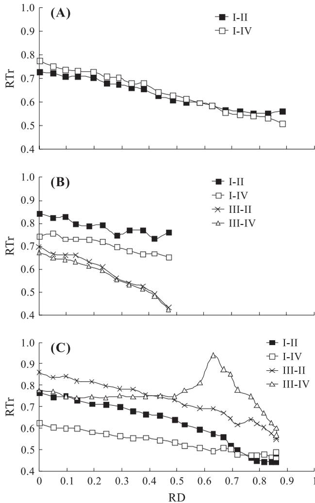
**Fig. 5.** Relationship of the relative transit time in the tangential direction to radial direction (RTr) and the relative hole diameter (RD) for (A) a disk with a central hole, (B) a disk with an off-center hole which located between the start sensor and the center of the disk, and (C) a disk with an off-center hole located in any one of the quadrants.
