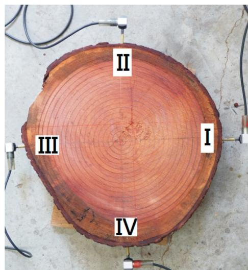
**Fig. 1. Setup of transit time detection by the stress wave device.**
