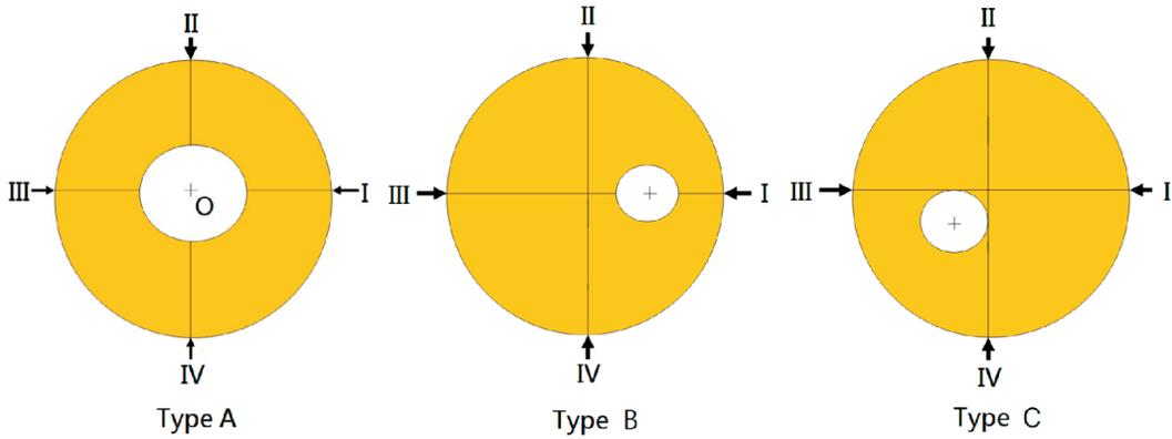
**Fig. 2.** Three types of hole positions in a disk. Type A, disk with a central hole; type B, disk with an off-center hole located between the start sensor and center of the disk; type C, disk with an off-center hole not located along any path among sensors.
