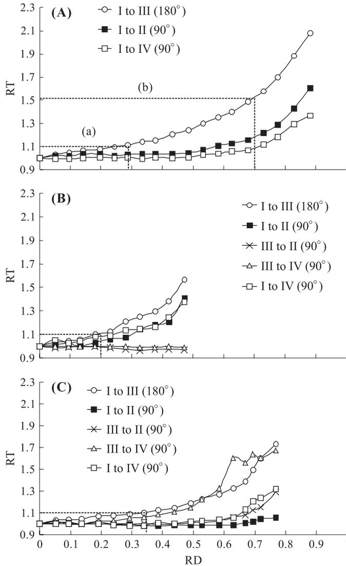
**Fig. 3. Relationship of the relative transit time for a disk with a hole to an intact disk (RT) and the relative hole diameter (RD) for (A) a disk with a central hole, (B) a disk with an off-center hole located between the start sensor and center of the disk, and (C) a disk with an off-center hole located in any one of the quadrants.**
