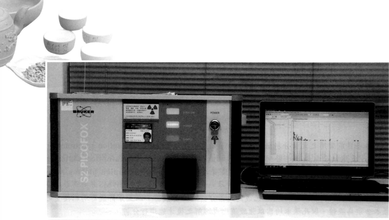
圖一、全反射式X光螢光光譜儀 (total-reflection x-ray fluorescence spectrometer, TXRF)
