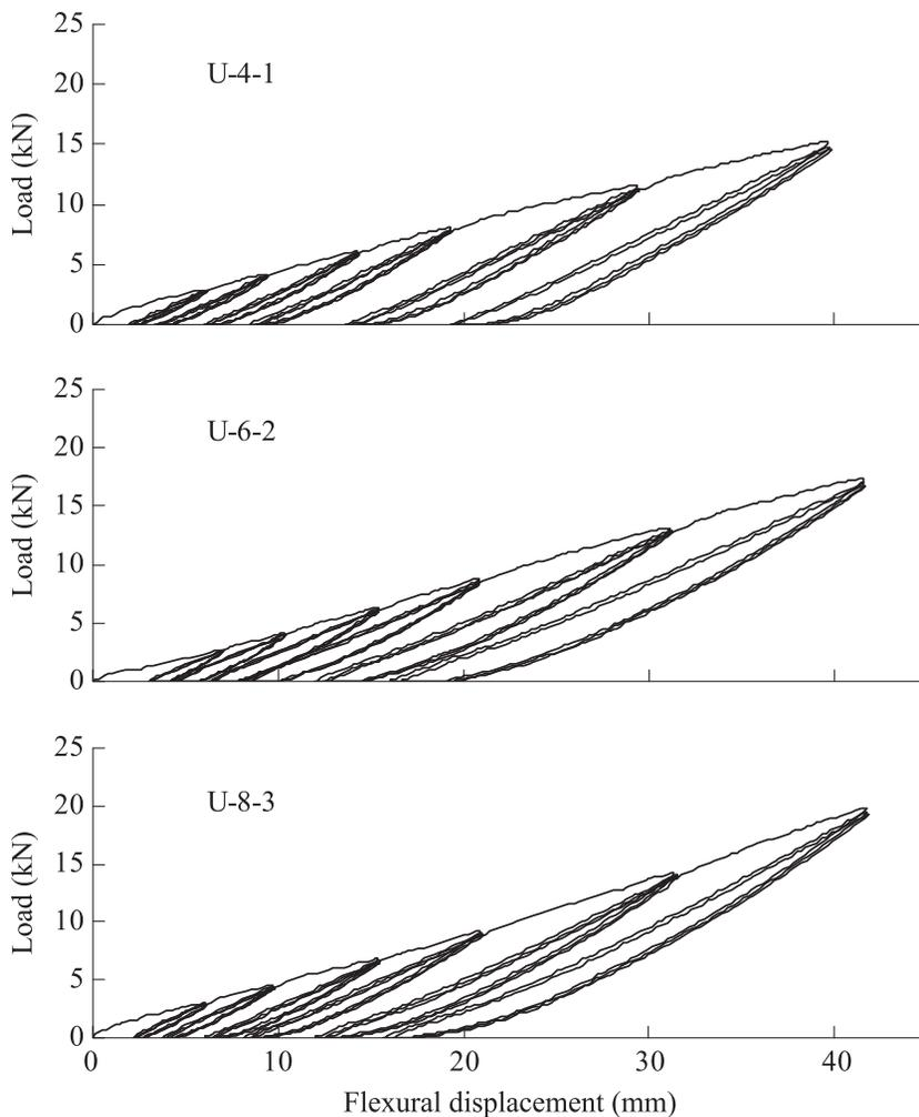
**Fig. 12.** Relationship between the load and flexural displacement of Japanese cedar glulam beams joined with U-type connectors subjected to a repeated loading application.
