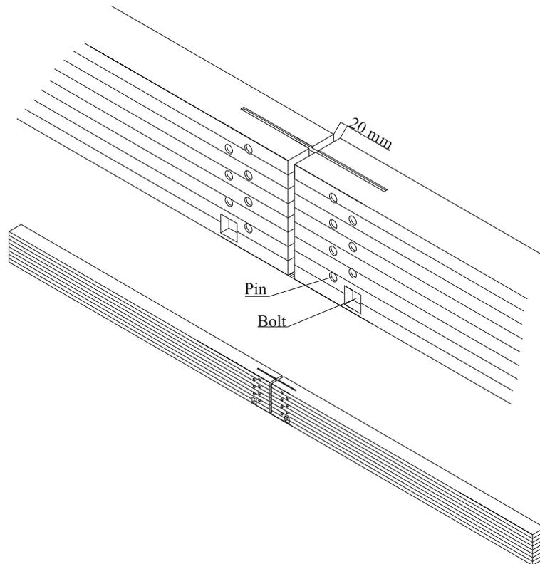
**Fig. 3. Schematic diagram of Japanese cedar glulam beam-to-beam connected longitudinally with the T-type metal connector. (8 embedded fasteners)**
