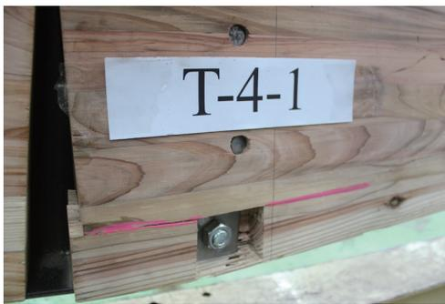
**Fig. 8.** Shear failure of middle-layer laminae at the bolt hole with a processed embedment.
