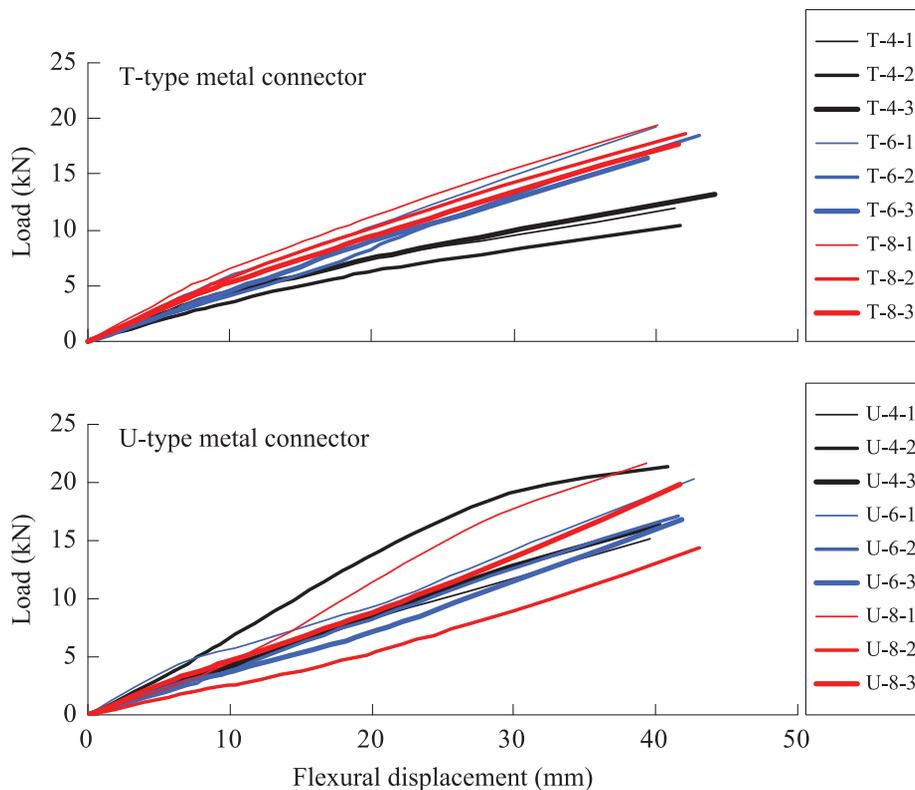
**Fig. 13. Initial envelop curves of Japanese cedar glulam beams connected with T- and U-type connectors subjected to repeated loading.**
