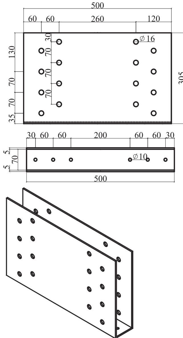
**Fig. 2. Design of U-type connectors for a Japanese cedar glulam beam-to-beam joint (8 fasteners). (unit: mm)**
