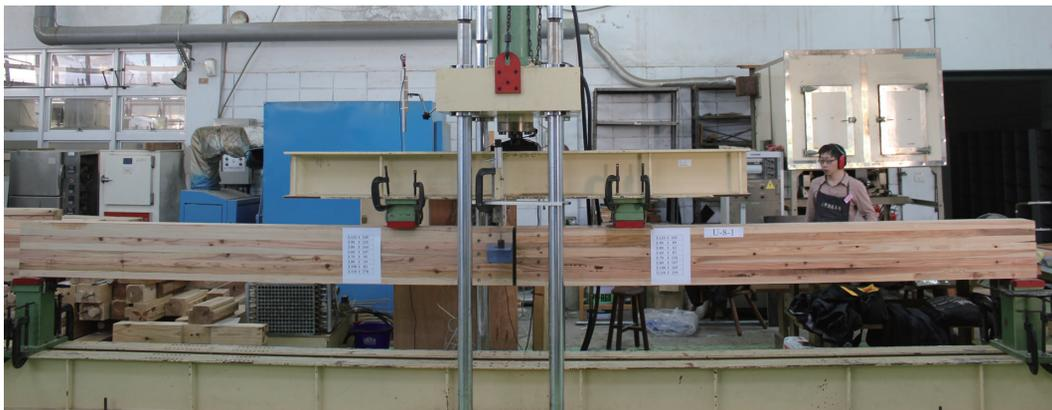
**Fig. 4. Four-point repeated bending test for Japanese cedar glulam member with a beam-to-beam U-type connection at the center.**
