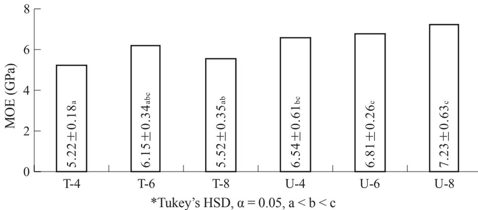
**Fig. 11. Modulus of elasticity (MOE) of end-to-end-connected Japanese cedar glulam beams with slotted metal connectors (T- and U-type) using different numbers of fasteners (4, 6, and 8).**
