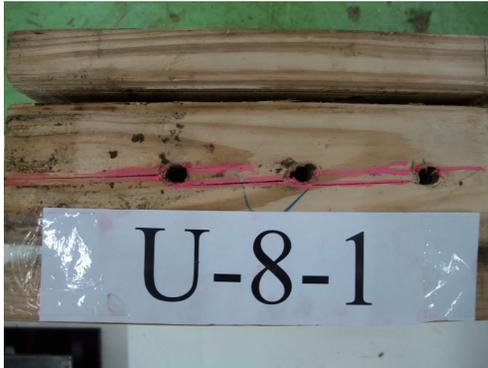
**Fig. 7.** After the connector and fasteners were removed, wood splitting was shown along the lag screw holes beneath the glulam member.
