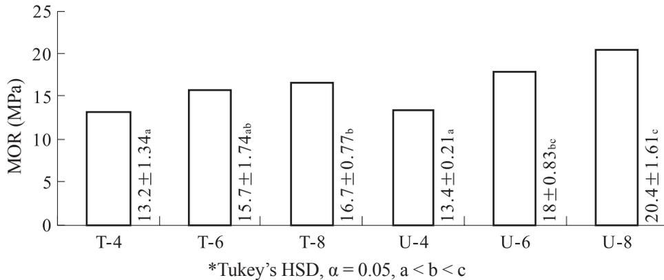
**Fig. 10. Modulus of rupture (MOR) of end-to-end-connected Japanese cedar glulam beams with slotted metal connectors (T- and U-type) using different numbers of fasteners (4, 6, and 8).**
