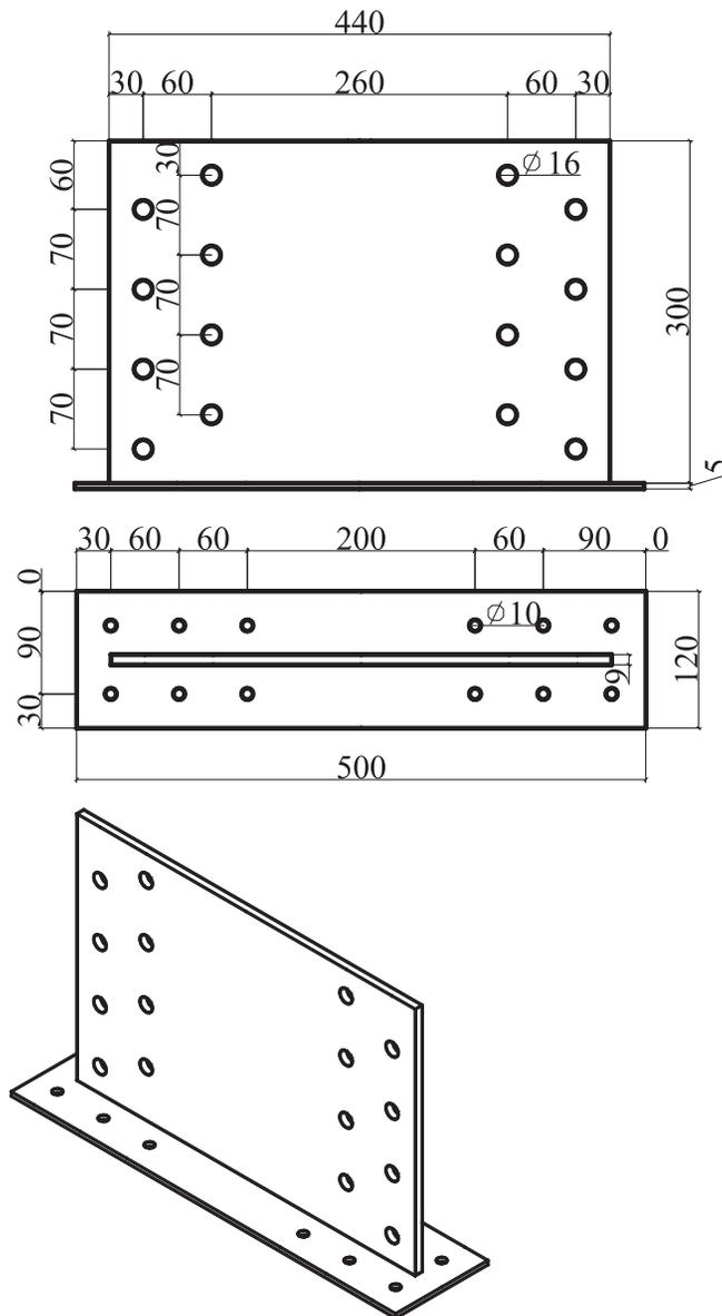
Fig. 1. Design of T-type connectors for a Japanese cedar glulam beam-beam joint (8 fasteners). (units: mm)
