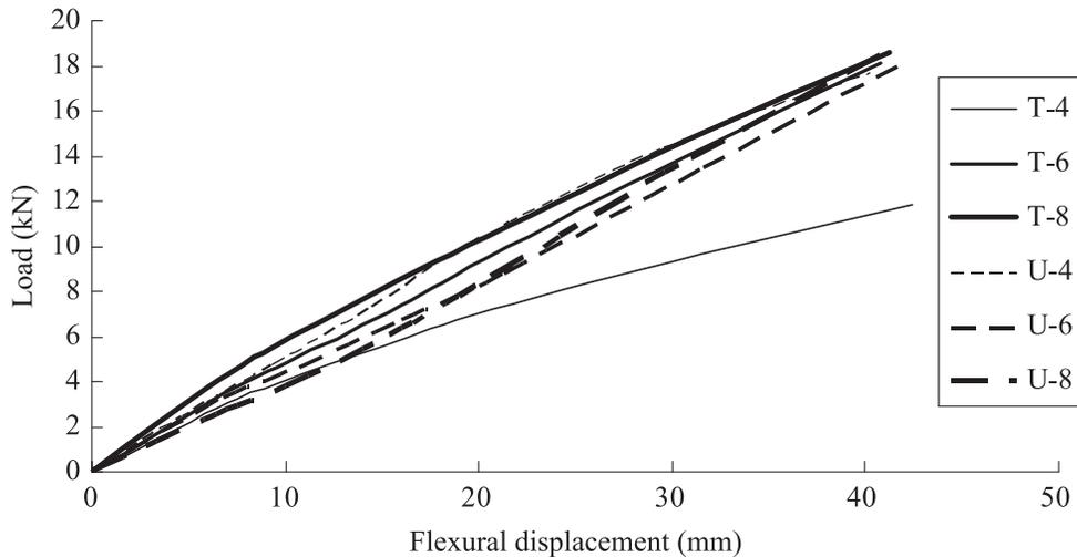
**Fig. 14. Stable envelop curves of beam-to-beam joints subjected to repeated loading for structural Japanese cedar glulam members.**
