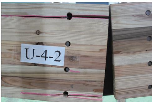
**Fig. 9.** Split at the outer laminae on both the top and bottom sides of the beam-to-beam connection.
