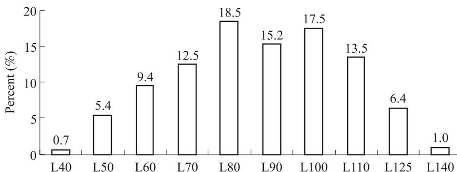
Fig. 6. Frequency distribution of the modulus of elasticity graded Japanese cedar laminae.
