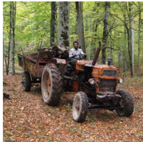
Fig. 1. UTB/Universal 650 farm tractor equipped with a 2-wheel trailer forwarding pulpwood from the forest in the study area.
