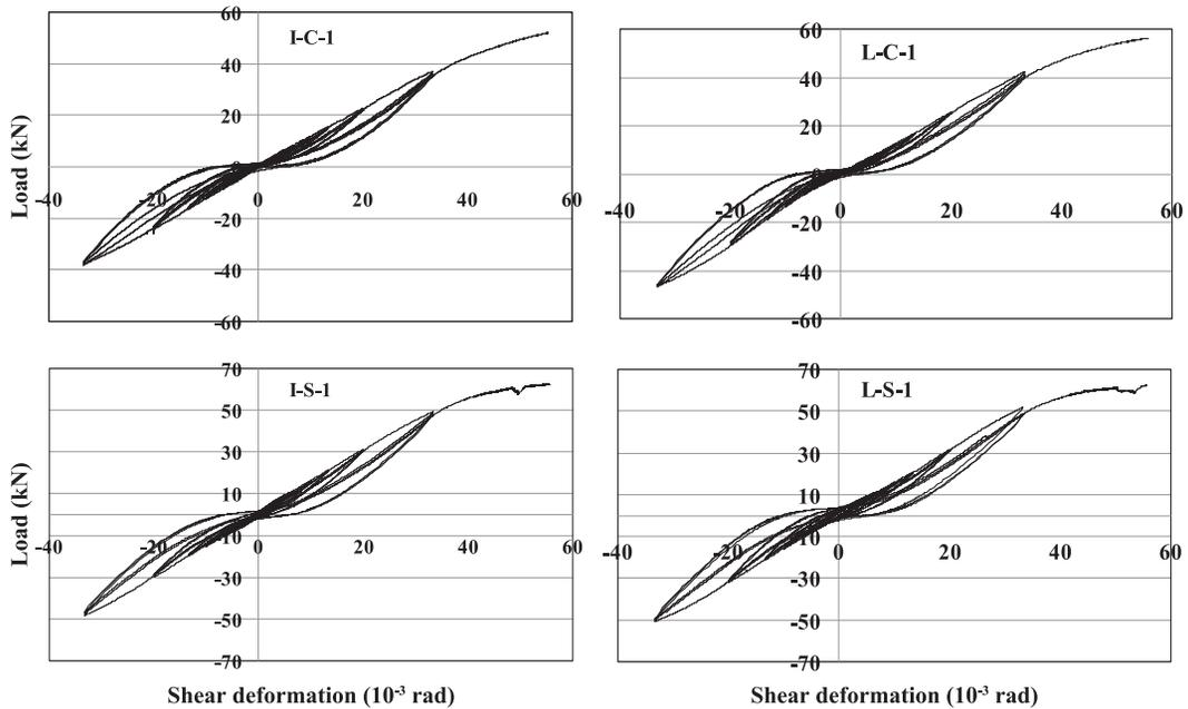
**Fig. 8.** Relationship between cyclic load and shear deformation of Japanese cedar portal frames jointed with I-C and I-S conditions. Conditions are illustrated in Figs. 2 and 3.
