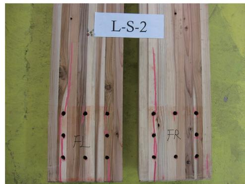
**Fig. 6. Splitting that occurred along bolted holes at the column base of a glulam portal frame during the racking test.**
