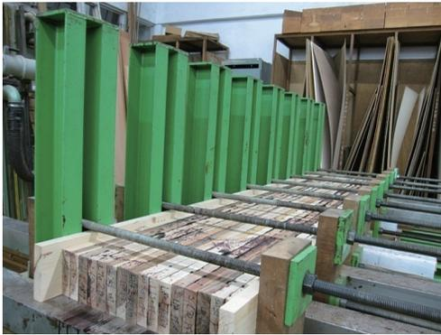
**Fig. 1.** Structural glulam assembled with Japanese cedar lamina after being glued and pressed.
