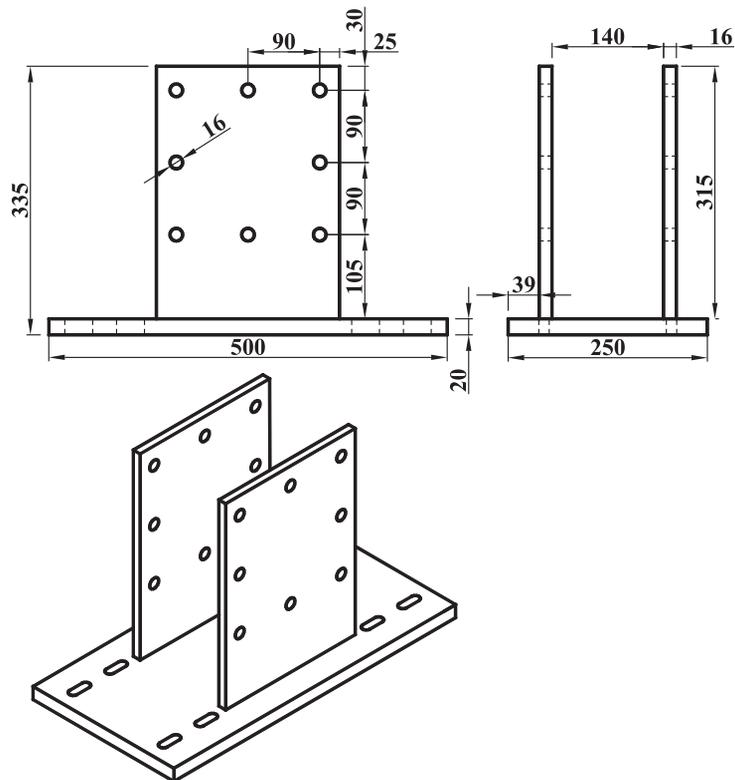
Fig. 4. Design of a mechanical connector for the column-base of a portal frame ( $\pi$  type) (units: mm).
