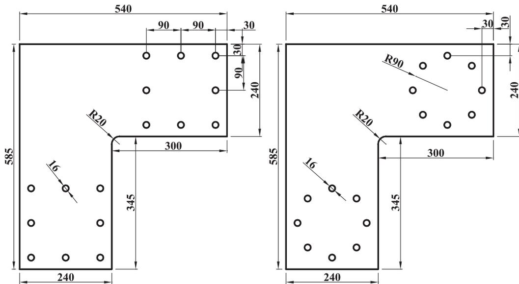
Fig. 3. Design of metal connectors for beam-column member joints in a glulam portal frame (L type) (units: mm).
