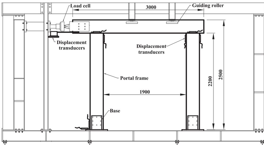
Fig. 5. Cyclic loading test for a portal frame structure assembled with Japanese cedar glulam members (units: mm).
