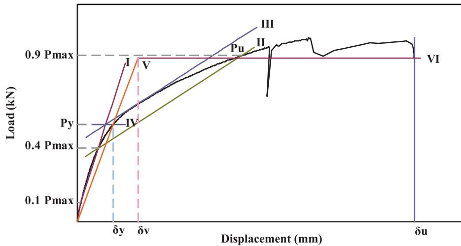
**Fig. 7. Demonstration on the evaluation of structural characteristic parameters for Japanese cedar glulam portal frames subjected to lateral loading (Yeh et al. 2012).**
