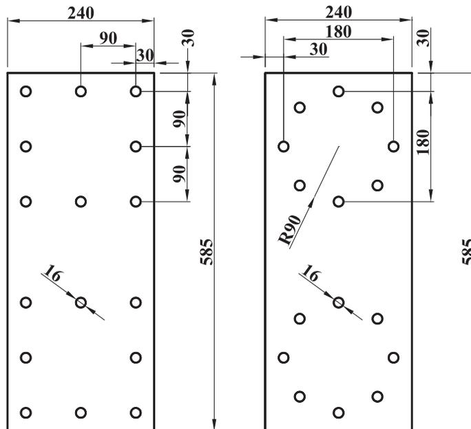
**Fig. 2.** Design of metal connectors for beam-column member joints in a glulam portal frame (I type) (units: mm).
