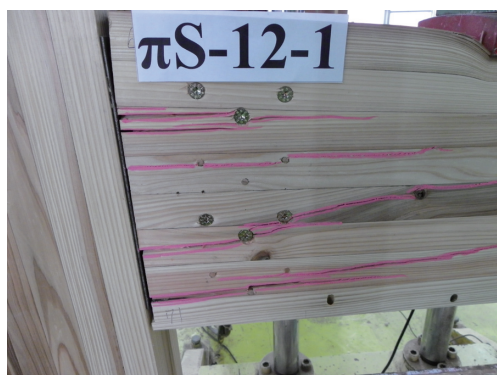
Fig. 8. T Wood splitting across a glulam beam section fastened with self-tapping screws.
