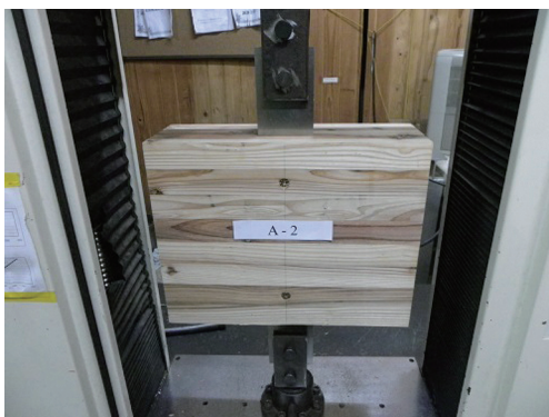
Fig. 7. Tensile test for the shearing strength of a single self-tapping screw through slotted steel/aluminum plates on a glulam member loaded perpendicular to the wood grain.
