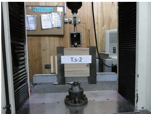
Fig. 6. Tensile test for the vertical withdrawal resistance of self-tapping screws from a glulam member.
