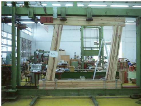
Fig. 8. Shear failure of a box-type glulam portal frame.
