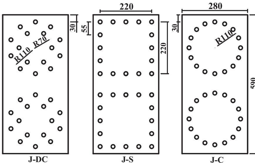
Fig. 1. Aluminum connectors with 3 types of self-tapping screw fastener arrangement. DC, double-circular; S, square; C, single circular.
