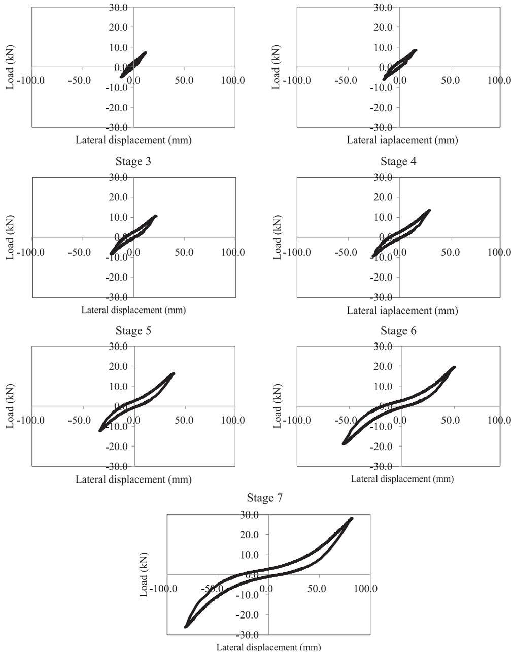
**Fig. 12. Energy dissipation in the third cycle of each cyclic load applied stage.**
