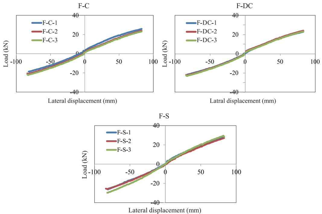
**Fig. 14.** Steady envelop curves of cyclic loading for boxed portal frames constructed with 3 different self-tapping screw arrangements. C, single-circular; DC, double-circular; S, square.
