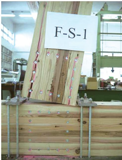
Fig. 7. Glulam column split along the fastener rows.
