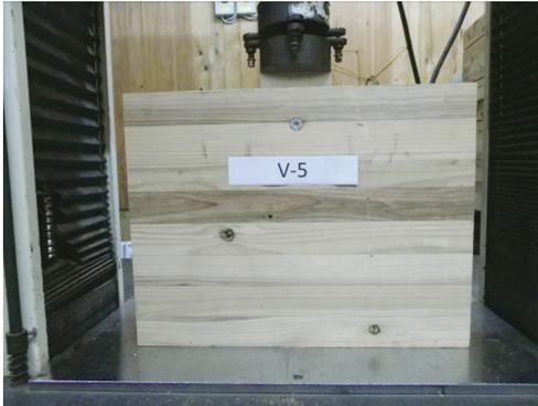
**Fig. 3.** Double shear strength of a self-tapping screw tested perpendicular to the wood grain.
