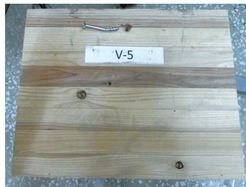
Fig. 9. Shearing off of a self-tapping screw by an aluminum plate in double shear testing perpendicular to the wood grain.
