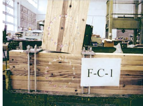
**Fig. 5.** Self-tapping screws indented into the wood surface in the racking test.
