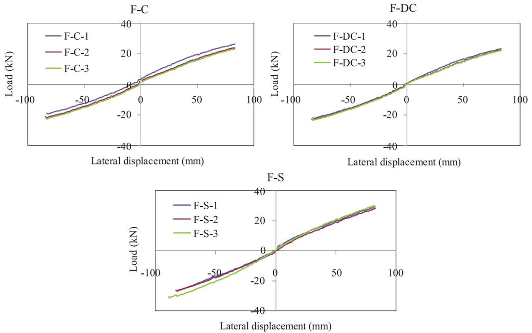
**Fig. 13.** Initial envelop curves of cyclic loading for boxed portal frames constructed with 3 different self-tapping screw arrangements. C, single-circular; DC, double-circular; S, square.
