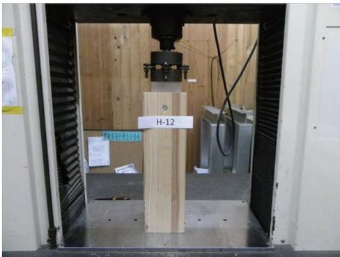
**Fig. 4.** Double shear strength of a self-tapping screw tested parallel to the wood grain.
