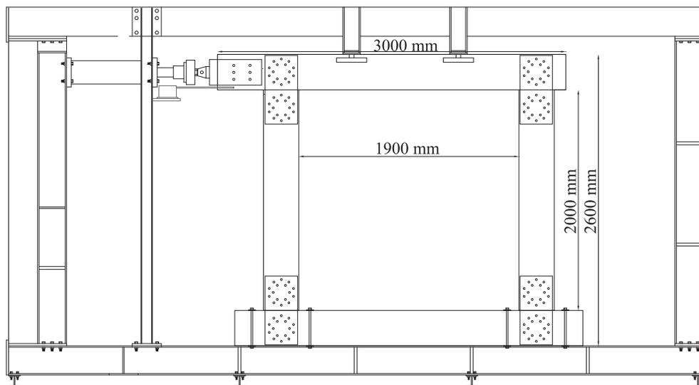
**Fig. 2. Racking test for a box-type portal frame constructed with Japanese cedar glulam.**
