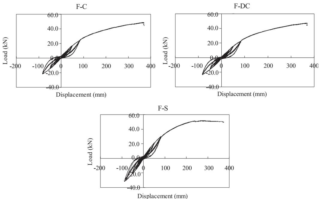
**Fig. 11.** Cyclic load-displacement relationship of portal frames fabricated with 3 different self-tapping screw placement patterns. C, single-circular; DC, double-circular; S, square.
