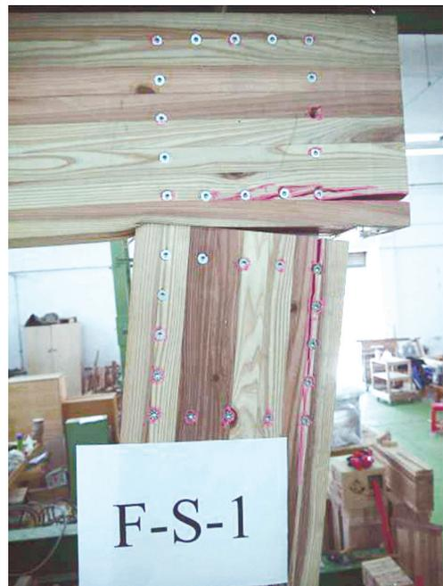
**Fig. 6.** Self-tapping screw head broken during the racking test.
