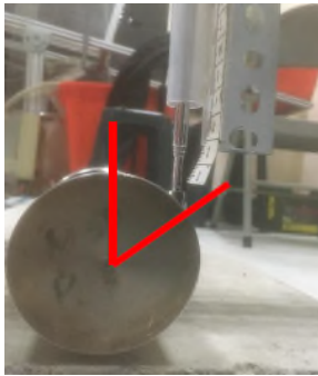
Fig.1 Steel ball free fall at 60°
