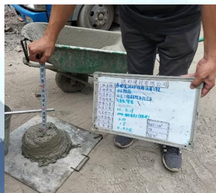
混凝土坍度試體試驗
