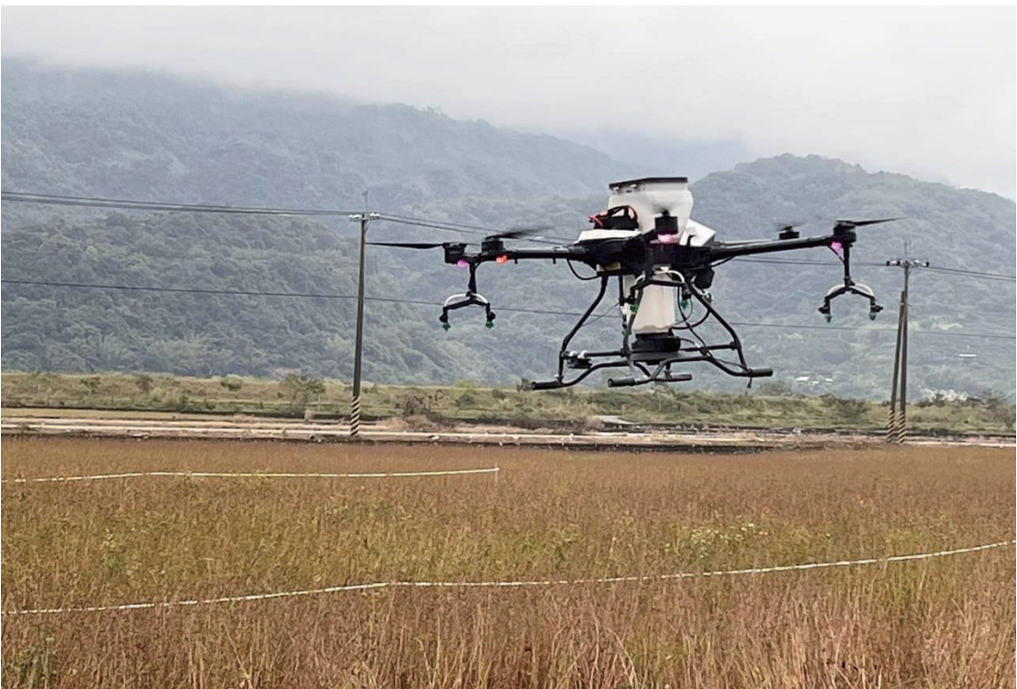
▲ 圖 4 無人機撒播蕎麥示意圖 Fig. 12 Illustration of buckwheat sowing by the drone.
