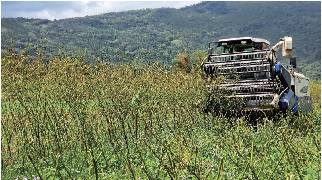
▲ 圖 3 雜糧聯合收穫機進行樹豆機械化採收 Fig. 11 Harvesting pigeon peas with a combine harvester.
