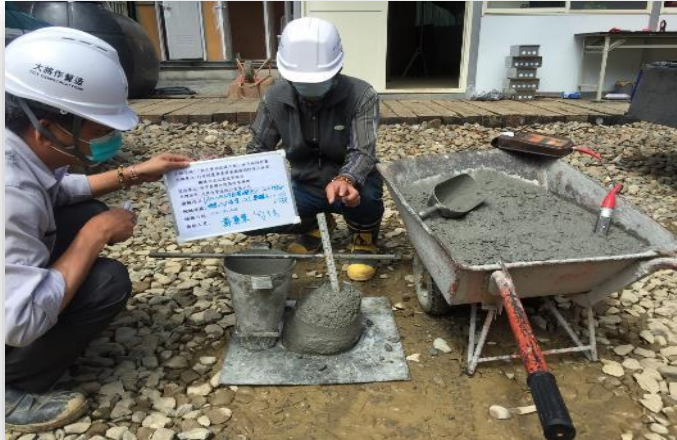
混凝土坍度試驗
