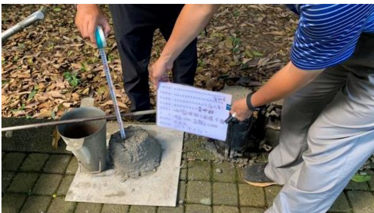
混凝土坍度試驗
