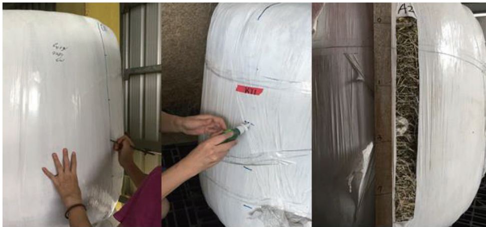
圖 1. 半乾青貯膠膜包的破損改善試驗。左：草包戳洞（ < 2 mm），中：藥劑處理與封孔，右：開封調查損壞比例。 Fig. 1. The damage improvement experiment of pangola grass haylage. Left: poking small holes ( < 2 mm) on haylage surface, Middle: reagent treatment and sealing, Right: investigation of damage situation.
