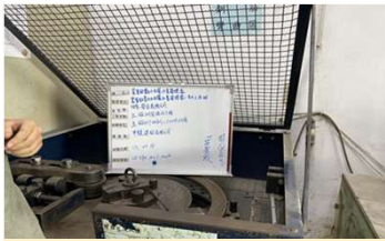
鋼筋彎曲試驗#3、#4
