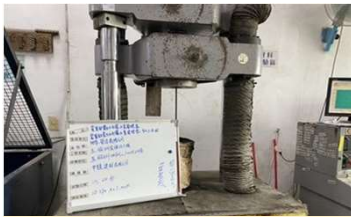
鋼筋抗拉試驗#3、#4
