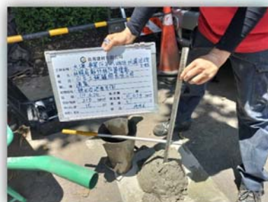
混凝土坍度試驗
