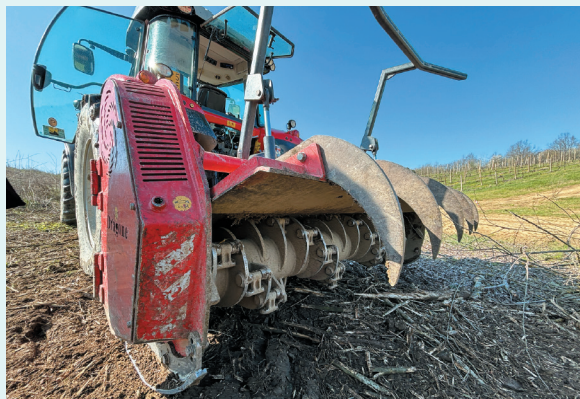
▲ 附掛式碎枝機特殊設計的強化鋼製迴轉刀軸可細碎果木枝條
