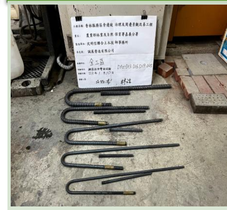
鋼筋抗拉、抗彎
