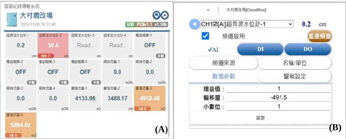
圖二、智慧灌溉系統開關水操作畫面(A)、水位計數值設定操作畫面(B)。 Fig. 2. Operation screen of the smart irrigation system's on/off water control (A) and the setting screen for the water level gauge (B).
