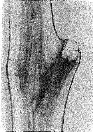
Fig. 5. The branch diameter as shown on the vertical section of an unpruned Taiwan zelkova stem is about 3.5 cm. The branch dried when the tree was 7-years-old; it persisted on tree stem for more than 2 years and, thus, formed dead knot.
